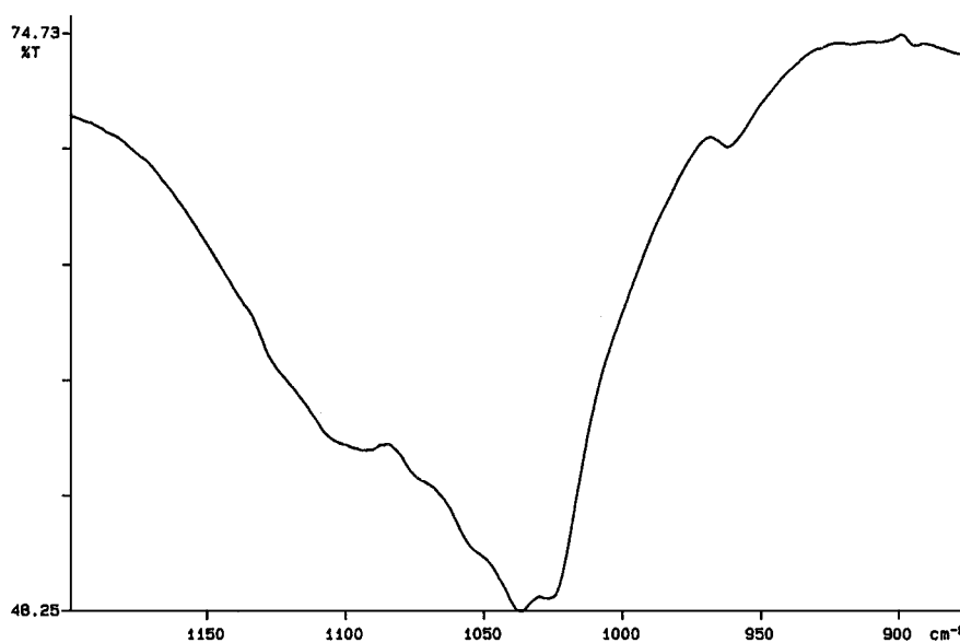
FIG. 5. IR spectrum of OCPam treated in a wet atmosphere at 40°C for 6 h.
